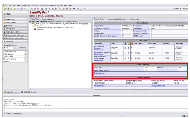
You can further analyze your logic utilization and register usage by examining the Log file looking at the Core Cell Usage section as shown below:
