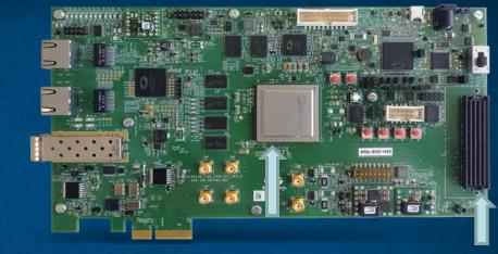
Using the PolarFire FPGA Eval kit and a custom PCB, benchmark various RISC-V core configurations in Triple Modular Redundancy (TMR) for use in NASA's Caution and Warning System (CWS) in the Portable Life Support System (PLSS) of the newest space suit (xEMU - Exploratory Extravehicular Mobility Unit).
