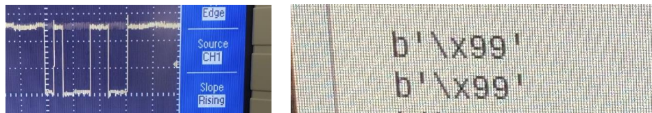
Figure 3 & 4: Left - Full Duplex Transmitting 0x31 at 1Mhz; Right - What was received, showing inaccuracy of Baud Value equation
